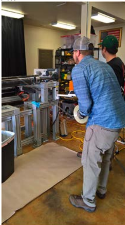
According to Composites One, filament winding is a suitable manufacturing process for the CSU rocket because it places fibers around the circumference of the tube to produce parts with high strength.
