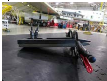
The first carbon fiber part 3D printed for the US Air Force: a first aid kit restraint strap for B-1 aircraft. (Photo courtesy Business Wire.)
