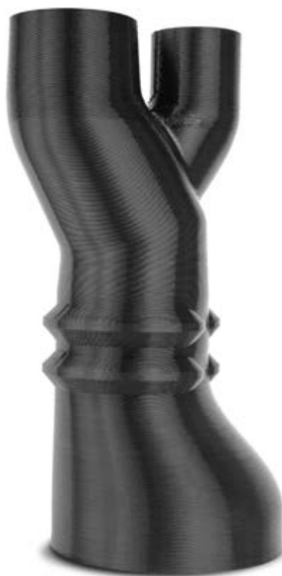
A 35 cm tall branched duct, 3D printed on a pellet printer with DuPont's Hytrel TPC-ET.
