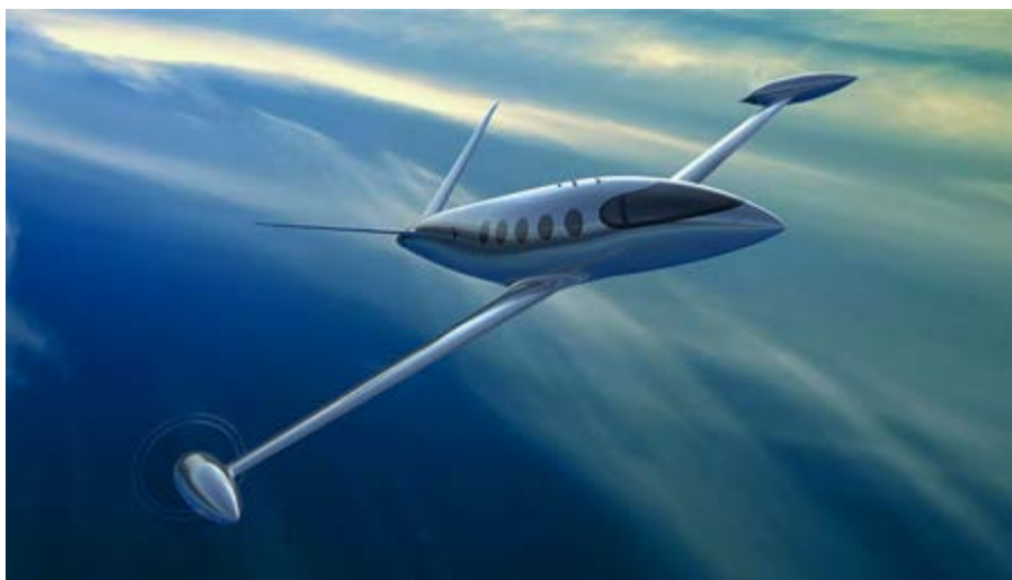
The Eviation Alice uses the lightest possible carbon fiber composite airframe.
